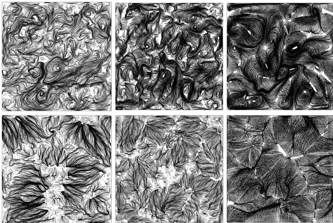
Fig. 8. Trajectories of massless particles of an instantaneous velocity field portraying the resolved flow structures in the central horizontal plane ( z/H = 0.5 ; above) and inside thermal boundary layer ( z/H = 10^{-3} ; below). Left: well-resolved LES. Middle: HYBRID. Right: T-RANS approach; Ra = 10^9 .
